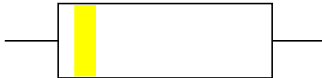
Figure 1: Resistor color codes: Black=0, Brown=1, Red=2, Orange=3, Yellow=4, Green=5, Blue=6, Violet=7, Gray=8, White=9.
